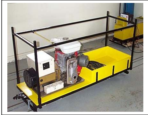
Work Trolley with Petrol Generator.
