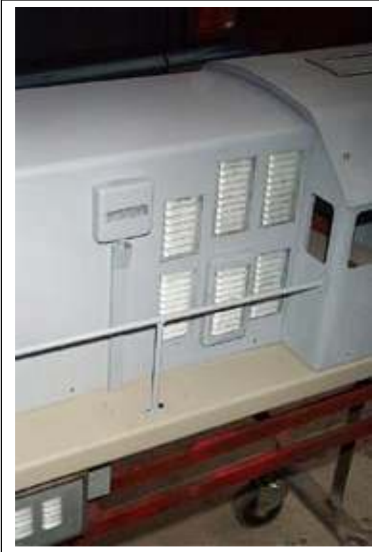
This view shows the louvers that a special punch was made to form.
