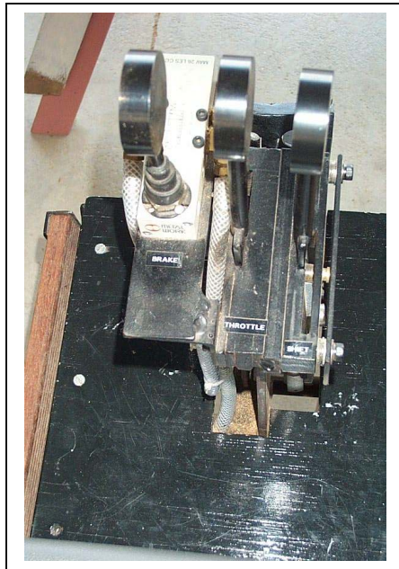
The three control levers. Left brake, centre throttle and right forward/reverse hydraulic control
