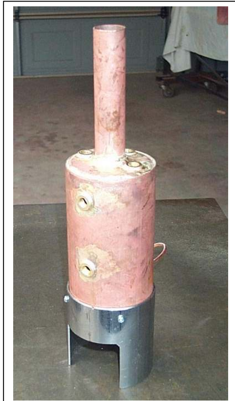
Crane Boiler ready for fittings
