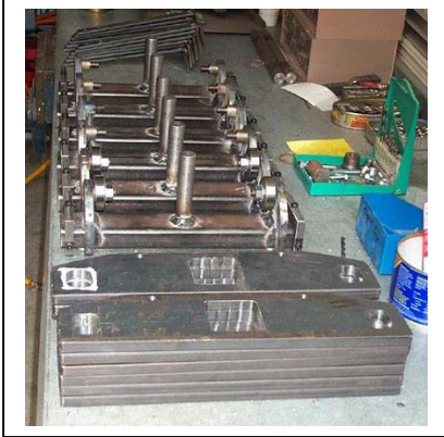
Bogie trunions and side plates ready for assembly.
