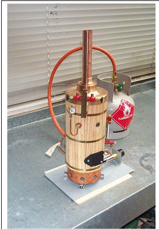
LPG fired vertical boiler made for friend
