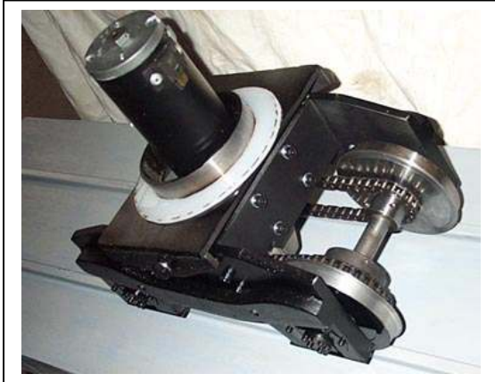
DH power bogie. Shows the motor mounted vertically through the trunion and pivot.
