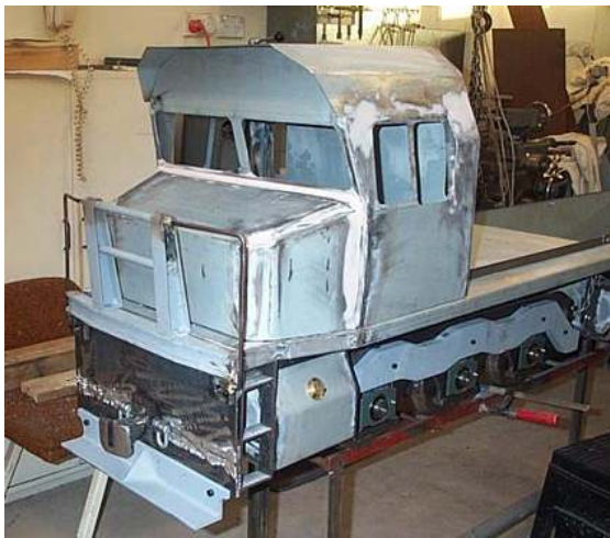
Built up cab structure for the DXR.
